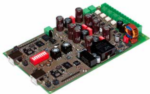
Computer- and Power Unit of acoustic subassembly
